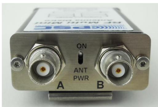
RF BNC Inputs Marked as “A” and “B”
