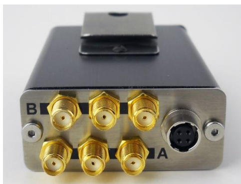
RF SMA outputs Marked as “A” and “B” Sides
