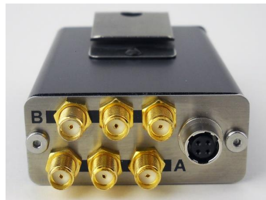
Bottom panel: SMA RF Outputs, Hirose
