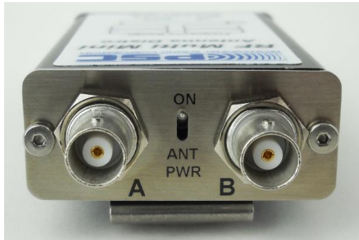
Top Panel: Power Switch, BNC RF Inputs
